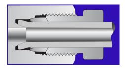
Flared cone connections create two high integrity metal-to-metal seals.
