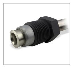
Flared cone connections on tube ends comprise just three components – the tube, a single compression sleeve and the gland nut.
